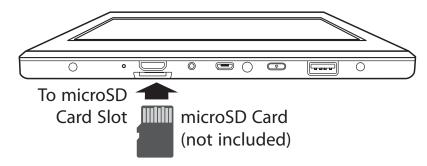
Insert the microSD card into the tablet's microSD slot until it clicks.
