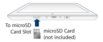
Insert the microSD card into the tablet's microSD slot until it clicks.
